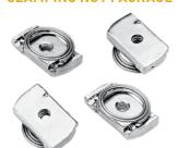
Twenty plated clamping nuts with top-grip nut retainers. Clamping nuts fit into mounting channels that are used on inside walls of Hoffman enclosures. Clamping nuts are included with all Hoffman accessories that attach to mounting channels. These clamping nuts can be used for mounting other equipment (brackets, etc.) to the enclosure walls.
